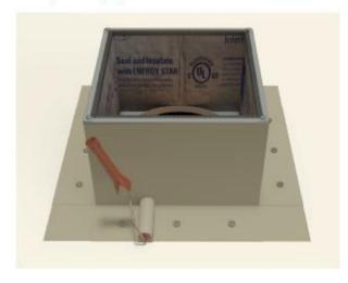
Step 11: Apply a generous amount of heat & pressure to TPO boot to weld it on to the curb & the deck.
